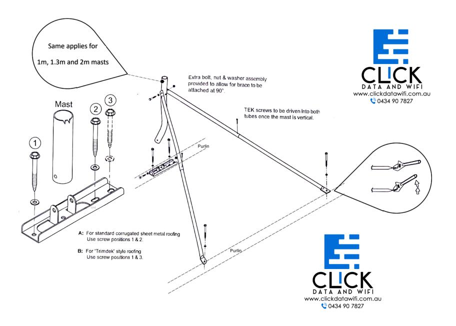
**Recommendation:** If practical, it is recommended to install the stay arms above the base mount coming down from a higher purlin. Opposite to the above diagram. This avoids length issues with the stay bars if the purlins are too widely spaced apart.
